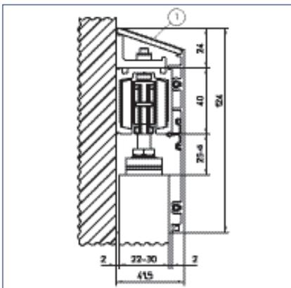
Clip-on cover, wall installation, wooden leaf 22-30 mm
