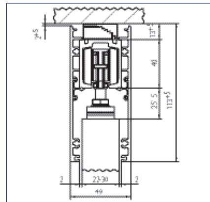
Clip-on cover, ceiling installation, wooden leaf 22-30 mm
