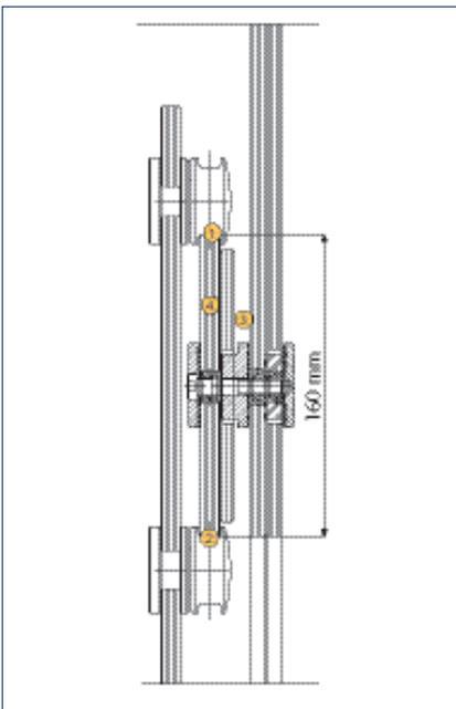
1. The plastic running surface of the stainless steel rollers, supported on ball bearings, slide almost noiselessly across the glass.
