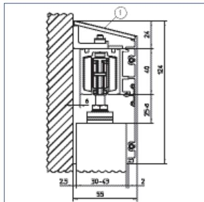
Clip-on cover, wall installation, wooden leaf 30-43 mm
