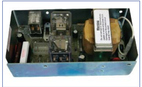
R411512 GT/SW Control Box
